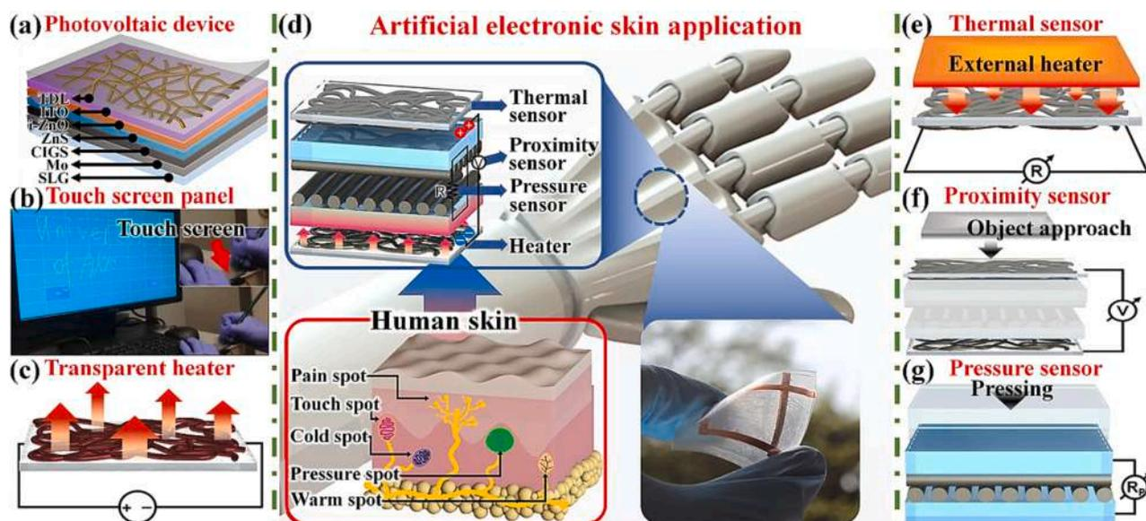
Fig. 11. Applications of TMFs as transparent conducting electrodes: (a) Photovoltaic devices [44] (©2019, Elsevier), (b) touchscreen panels [143] (©2014, American Chemical Society) (c) heaters, (d) e-skin, (e-g) thermal, proximity and pressure sensors for health monitoring [52] (© 2020, Springer Nature).
